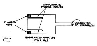
Fig. 2 - Moving-iron balanced-armature receiver element
