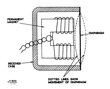
Fig. 1 - Moving-iron diaphragm receiver element
