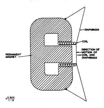
Fig. 3 - Moving-coil receiver element
