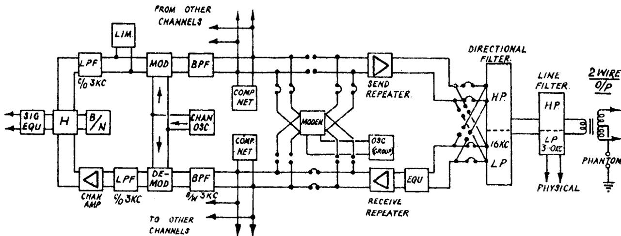
Fig. 11. Block schematic diagram of two-wire terminal.
