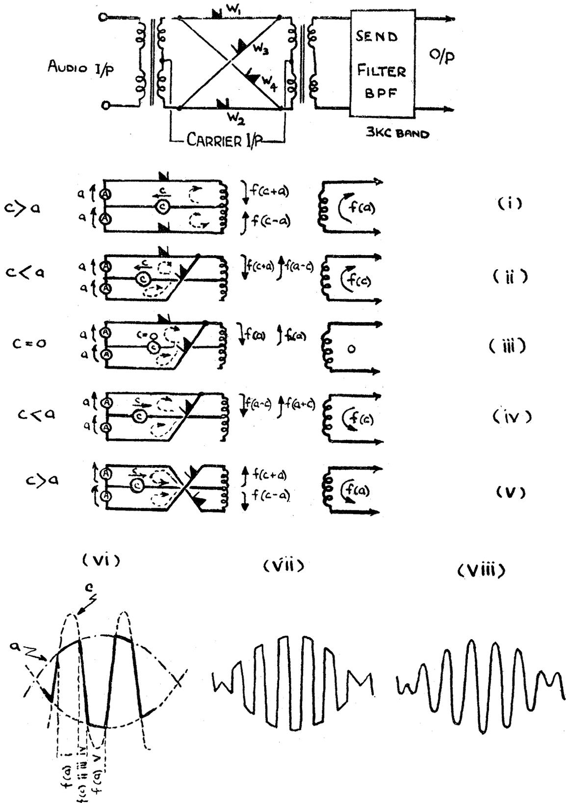
Fig. 4. Action of rectifiers in modulation.
