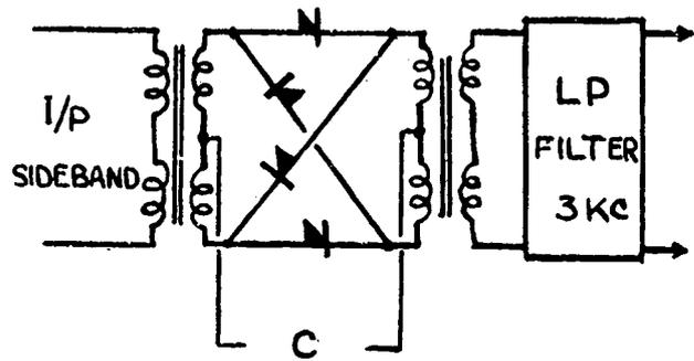
Fig. 5. Skeleton circuit showing principles of demodulation.
