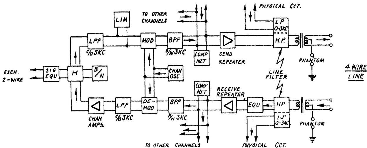
Fig. 10. Block schematic diagram of four-wire terminal.
