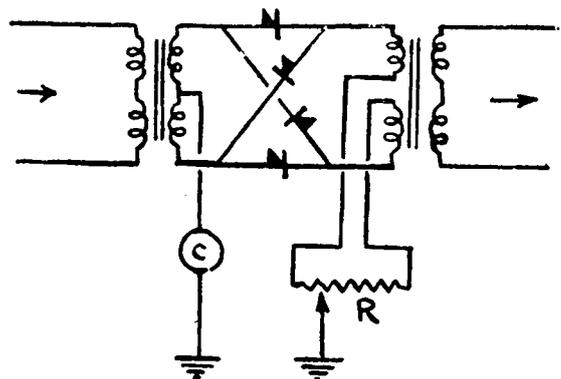
Fig. 7. Carrier leak potentiometer.
