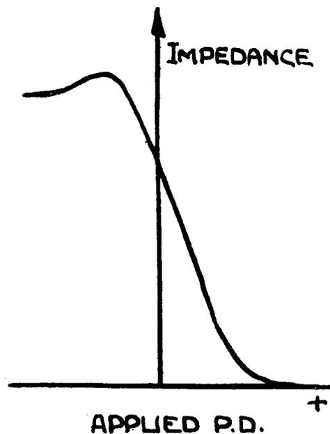
Fig. 6. Characteristic of copper oxide rectifier.
