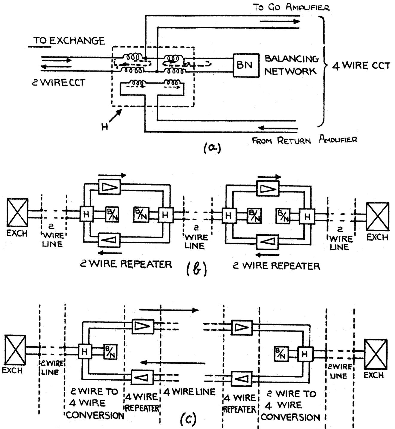
Fig. 1. (a) Two-wire to four-wire conversion (hybrid) system.
