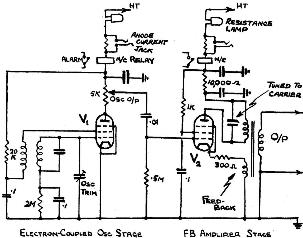
Fig. 9. Channel oscillator.
