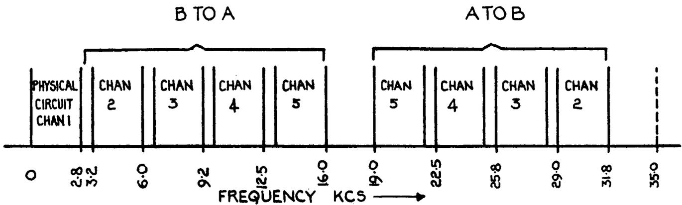
Fig. 3. Diagram of channels in frequency spectrum of Army 1 + 4 carrier system working two-wire.
