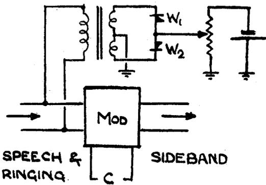
Fig. 8. Automatic limiter circuit for 500 c/s signalling tone.
