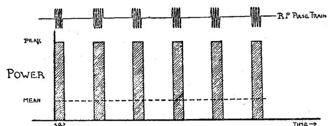
**PEAK AND MEAN POWER.** IN THE ABOVE DIAGRAM AN R.F. PULSE TRAIN AND THE POWER-TIME DISTRIBUTION IN THE TRAIN ARE PLOTTED ON THE SAME TIME-SCALE. THE MEAN POWER OF THE TRAIN IS ALSO SHOWN, AND THE DOTTED LINE REPRESENTING THIS MEAN LEVEL CLEARLY MUST ENCLOSE WITH THE ABSCISSA THE SAME AREA FOR AN INTEGRAL NUMBER OF PERIODS  $T$  AS IS ENCLOSED IN THE SHADED RECTANGLES INCLUDED IN THIS NUMBER OF PERIODS. IT IS ALSO EVIDENT THAT FOR ANY SIMILAR PULSE TRAIN
