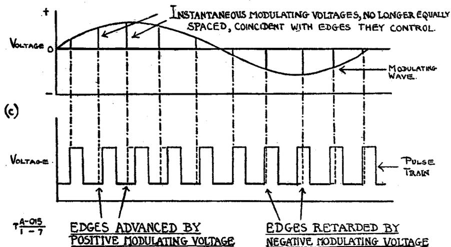
Fig. 7—Method of control of pulse width by modulation voltage
