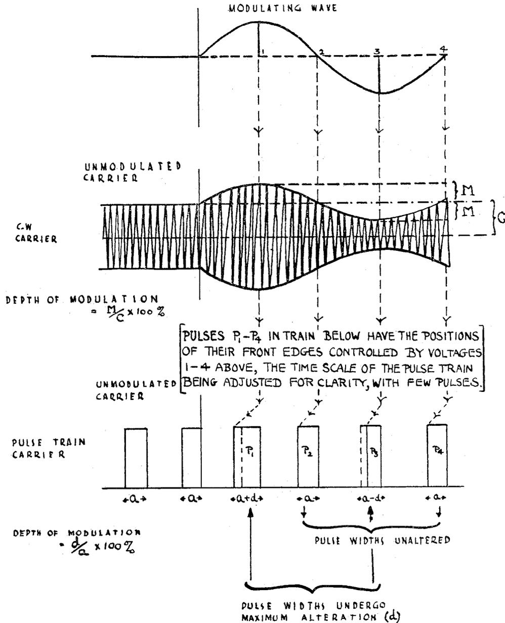
NOTE:- THE DIAGRAMS SHOW THE RESULTS OF MODULATION OF A SINE CARRIER AND A PULSE TRAIN BY A MODULATING WAVE. THE AMPLITUDE OF THIS MODULATING WAVE IS THE GREATEST ENVISAGED IN THE SYSTEM FOR ANY FREQUENCY THE EXPRESSION DEPTH OF MODULATION, FOR WHICH VALUES ARE DERIVED ABOVE, INFERS MAXIMUM MODULATING VOLTAGE.
