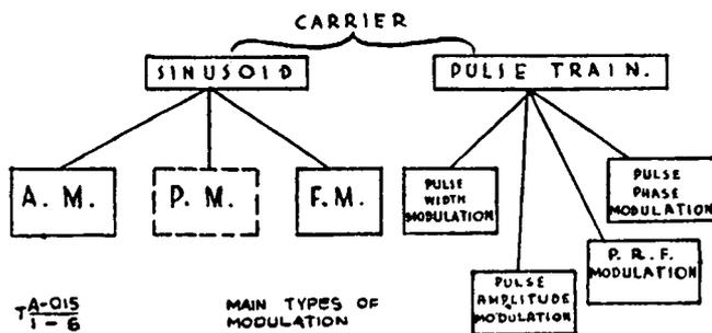
Fig. 6—Main types of modulation
