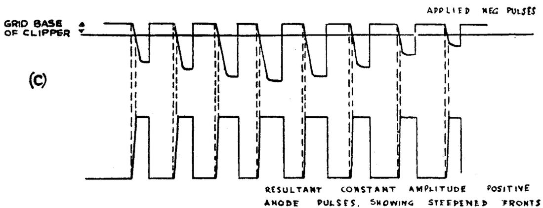
ILLUSTRATING THE EFFECTS OF THE CLIPPING PROCESS IN PRODUCING
