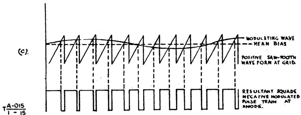
ILLUSTRATING PROCESS OF WIDTH MODULATING A 10k c/s PULSE CARRIER WITH 1k c/s INTELLIGENCE
