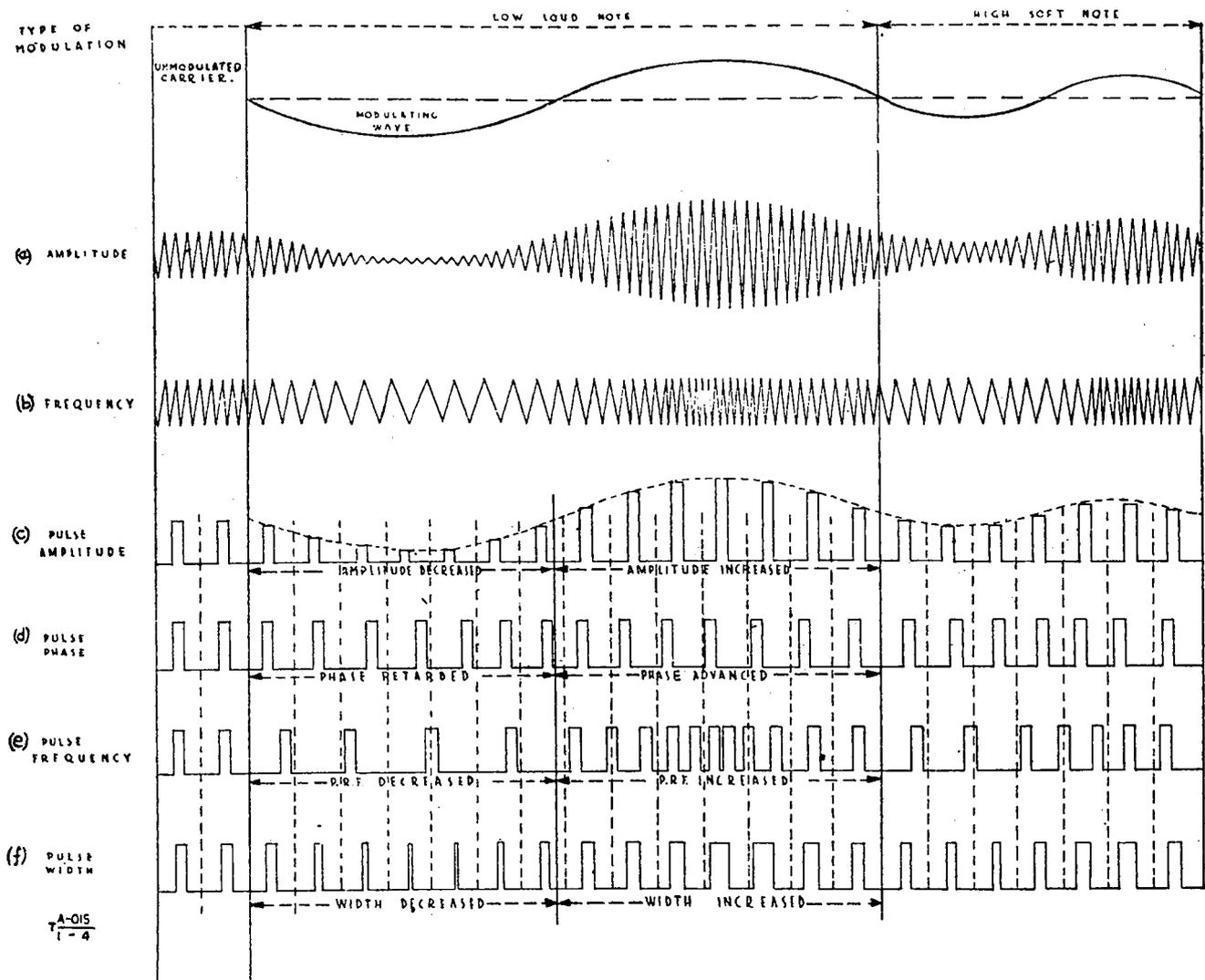
Fig. 4—Diagrammatic representation of different types of modulation
