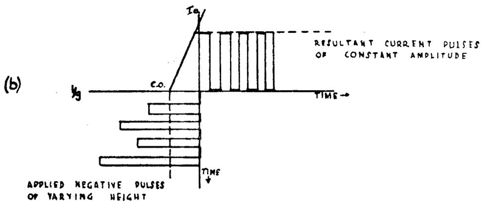
THE CLIPPING PROCESS ILLUSTRATED BY REFERRING THE APPLIED AND RESULTANT WAVEFORM TO THE (DYNAMIC)  $I_a - V_{g_2}$  VALVE CHARACTERISTIC
