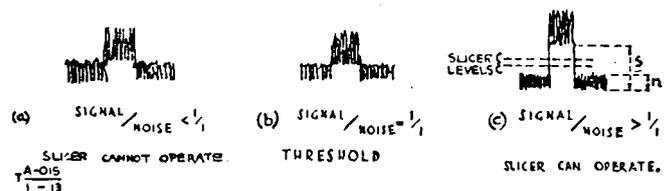
Fig. 13—Ratio necessary for operation of slicer
