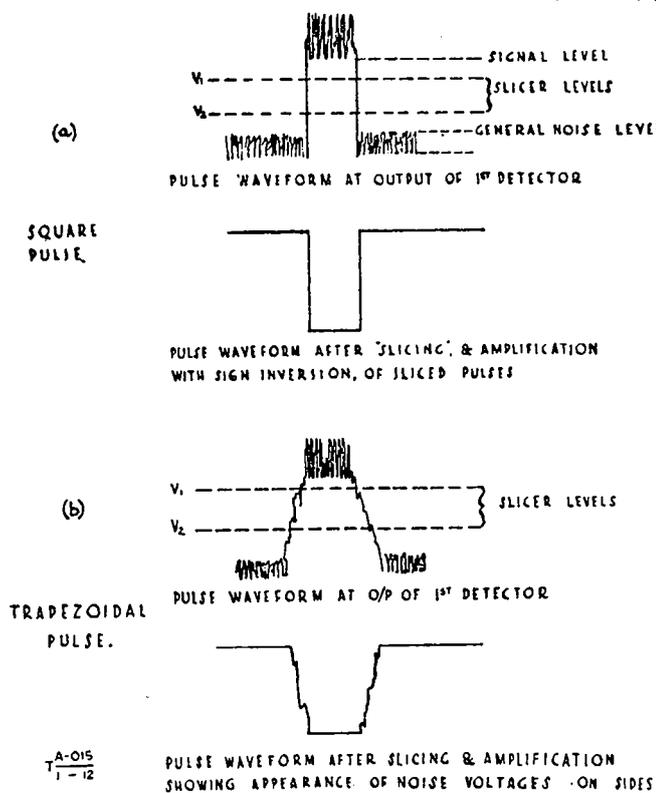
Fig. 12—Operation of slicer
