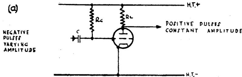
BASIC CIRCUIT FOR CLIPPING NEGATIVE PULSES
