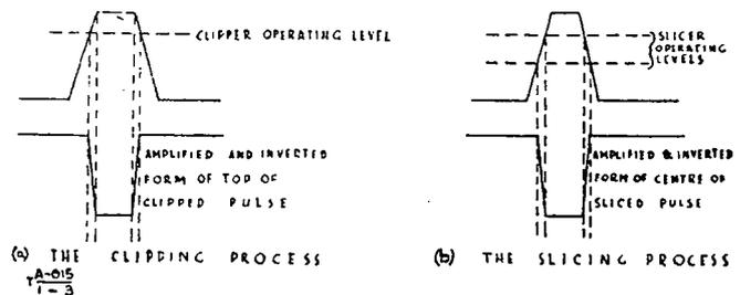
Fig. 3—Pulse clipping and slicing
