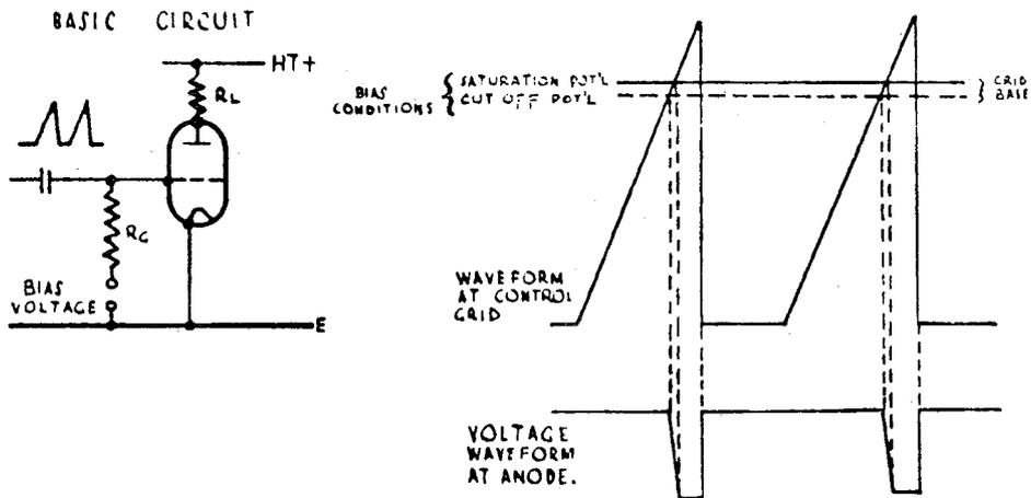
(a) SHOWING GENERATION OF APPROX. SQUARE NEGATIVE PULSES AT ANODE OF VALVE HAVING SHORT GRID BASE
