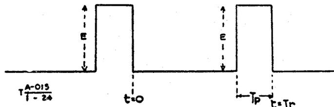
Fig. 24—Train of rectangular pulses
