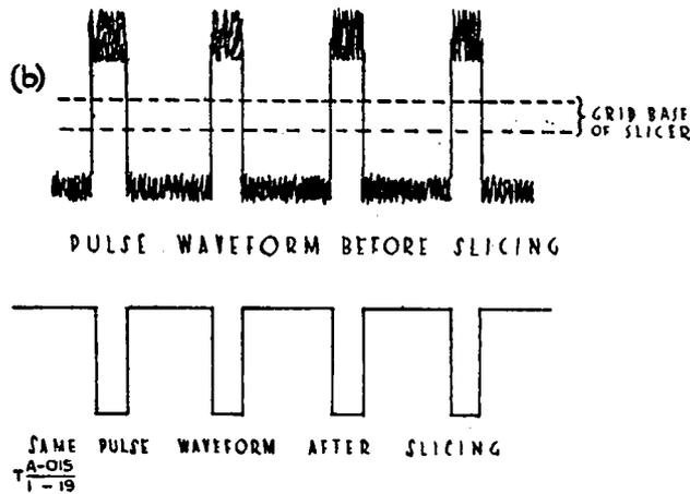
Fig. 19—Application of slicing circuit
