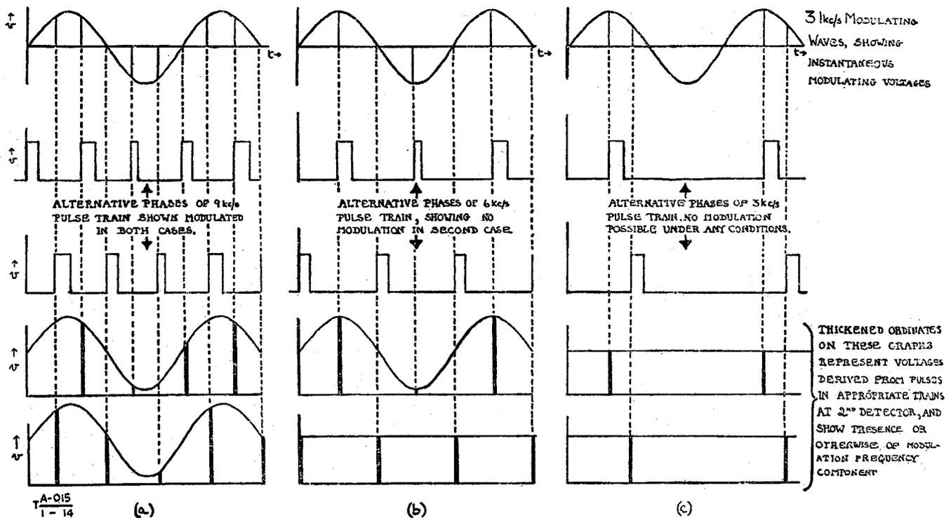
Fig. 14—Diagram showing results when carrier frequency approaches modulation frequency
