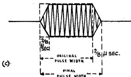
FORM OF ORIGINALLY IDEAL PULSE, AFTER PASSAGE THROUGH IF. CIRCUITS WHOSE BANDWIDTH IS B WHERE B IS CHOSEN TO PASS MAJOR PART OF PULSE ENERGY CONTENT
