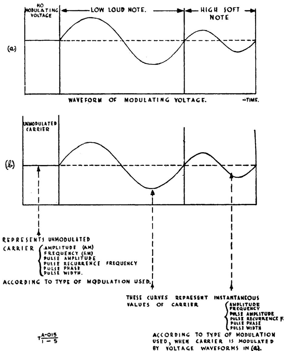
Fig. 5—Linear modulation of a carrier
