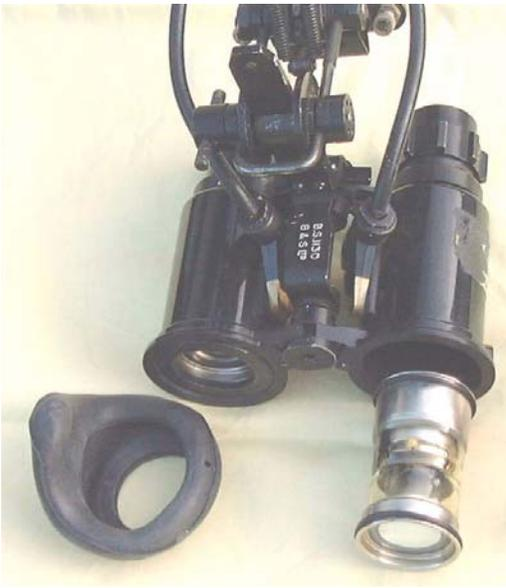
*Binoculars partially dismantled showing the image converter removed which measures 2.25 inches long and 1.4 inches wide*
