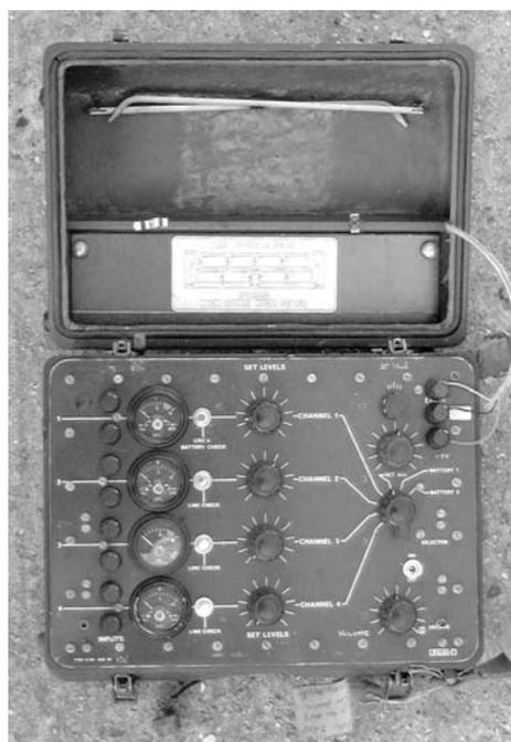
*TOBIAS Mk1. Note the flimsy aluminium stays carried in the lid housing the battery box beneath. The delicate cable feed was attached to the main unit via terminals on the right hand side.*
