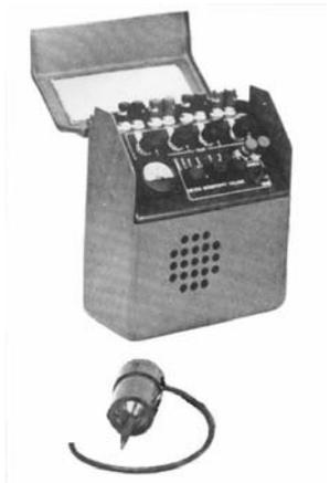
*Texas X150A control unit measuring 7 x 4 x 9 inches shown with one seismometer.*
