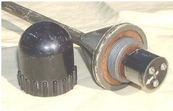
*The 'Tyril' dome removed showing the sensor head. Note the arrow allowing alignment with the front of the tank.*
