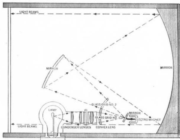
On transmit, the signal from the microphone was amplified and caused an electromagnetic to vibrate a mirror, in a similar way to Bell's photophone. Light from an electric lamp was focussed into a beam of light directed onto this mirror reflecting the light beam in proportion to the speech. Further focussing by parabolic mirrors beamed the light through an infra-red filter to render it invisible to the eye.
