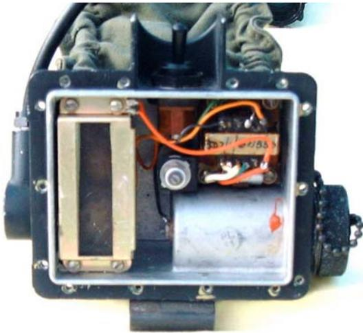
*The very compact power unit. To the lower right is the battery container, above that the single transistor and transformer, and to the left is the voltage multiplier unit. In the centre is a potentiometer to provide adjustment of the output voltage.*
