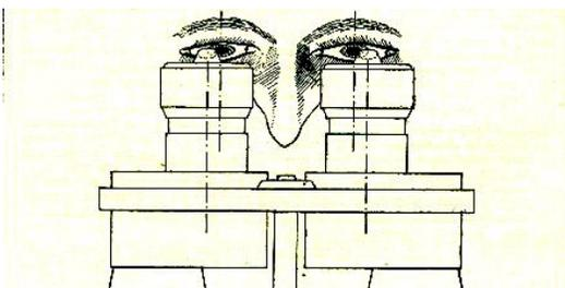
*Interocular setting is too wide, some of the light passing through the binoculars does not pass through the pupil and enter the eye, this makes the target appear dimmer or it may not be seen at all.*
