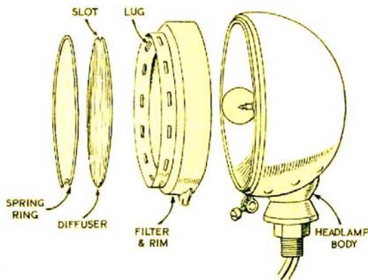
The filter gets hot, as it has to absorb all the white light energy. To avoid the plastic diffuser from melting, it is spaced from the filter by means of lugs. The holes, from which the lugs are formed, allow for some cooling unfortunately the lack support from behind the diffuser, means it can easily break.
