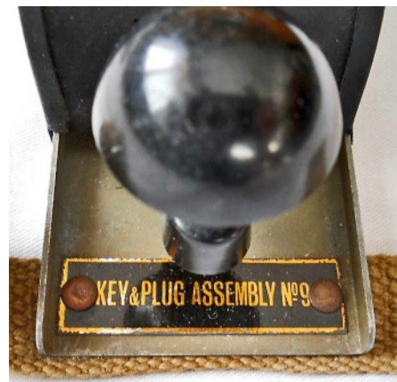
Internal view of Key and Plug Assembly No. 9 ver. 3.3 with Key W.T. 8 Amp No. 2 Mk.III (left) and front view showing the lacquered identification plate.
