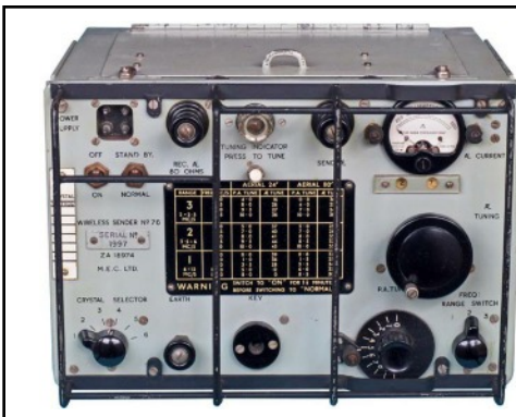
Wireless Set (or Sender) No. 76 was a portable transmitter developed in 1943. Use: light-weight self-contained transmitter for rear link communication. Frequency range 2-12MHz. RF output 9W. Crystal control. CW only. Range over 300 miles. It was normally used in conjunction with Reception Set R109A.
