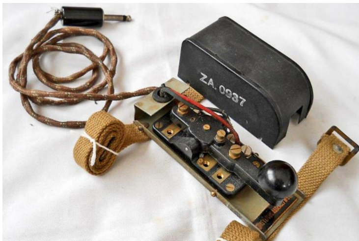
Internal view of Key and Plug Assembly No. 9 ver. 3.3 with Key W.T. 8 Amp No. 2 Mk.III (left) and front view showing the lacquered identification plate.
