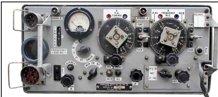
Wireless Set No. 19 Mk.II produced by RCA in the USA. Use: primarily developed for AFVs but later used as a general purpose set. Frequency range 'A' set 2-8MHz; 'B' set 229-241MHz. MO control. R/T, MCW, CW. RF output 'A' set 1.2-2.5W (R/T). Range 'A' set up to 15 miles; 'B' set 3/4 mile.
