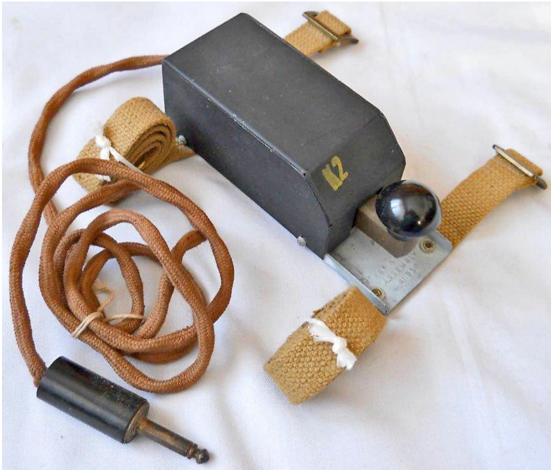
Key and Plug Assembly Cdn No. 9 Type 1.
