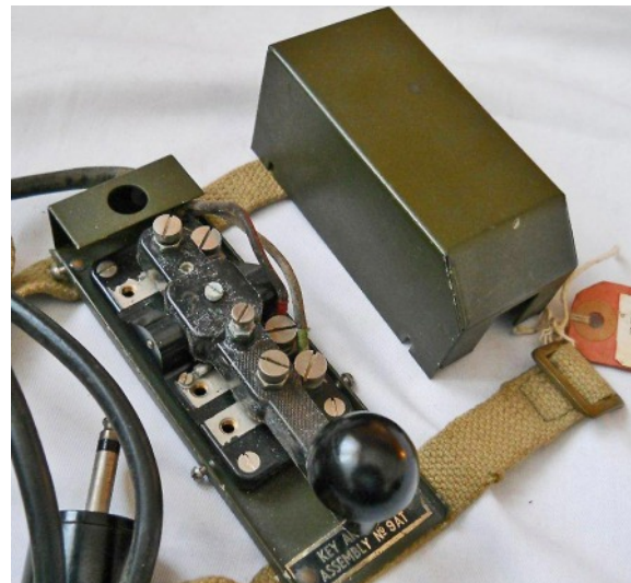
Key and Plug Assembly No. 9AT was a tropicalised version of ver. 4.1 and almost identical to ver. 4.3.
