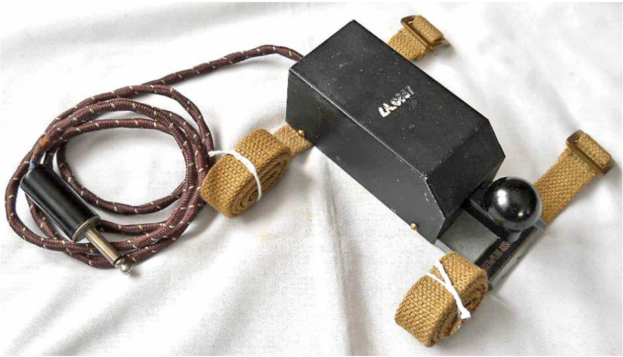
General view of Key and Plug Assembly No. 9 ver. 3.1.
