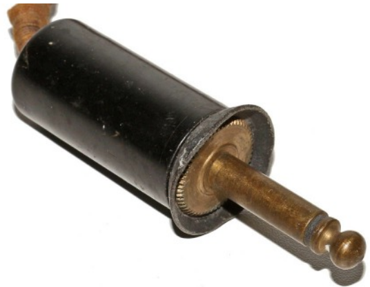
A black fibre disk protected the operator from coming into contact with high tension when inserting the key into the set key socket (above). This was an addition which was occasionally found fitted on other versions.
