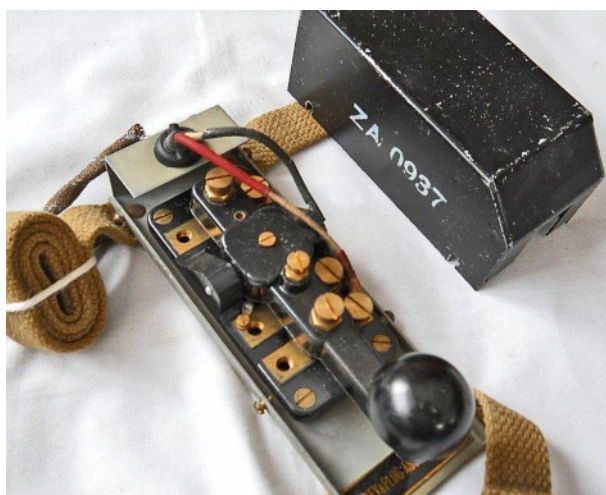
Key and Plug Assembly No. 9 ver. 3.2 with protective cover removed showing a Key W.T. 8 Amp No. 2 Mk.III (left). Detail view of the front with key knob and identification plate (right).
