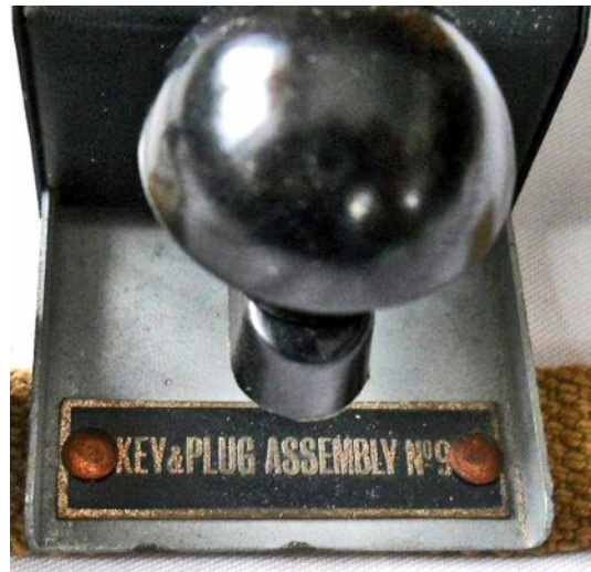
Internal view of Key and Plug Assembly No. 9 ver. 3.1 showing a Key W.T. 8 Amp No. 2 Mk.III. The difference between Key and Plug Assembly No. 9 ver. 3.1 and ver. 3.2 was only a unlacquered identification plate. The differences in the Morse keys were not taken in account.
