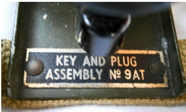
Key and Plug Assembly No. 9AT was a tropicalised version of ver. 4.1 and almost identical to ver. 4.3.
