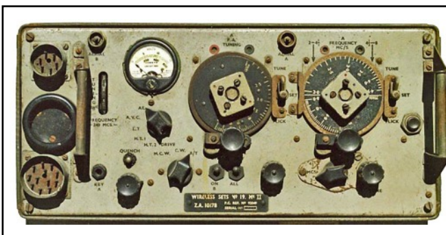
Wireless Set No. 19 (here shown the British Mk.II model, set without power supply unit). Use: primarily developed for AFVs but later used as a general purpose set. Frequency range 'A' set 2-8MHz; 'B' set 229-241MHz. MO control. R/T, MCW, CW. RF output 'A' set 1.2-2.5W (R/T). Range 'A' set up to 15 miles; 'B' set 3/4 mile.
