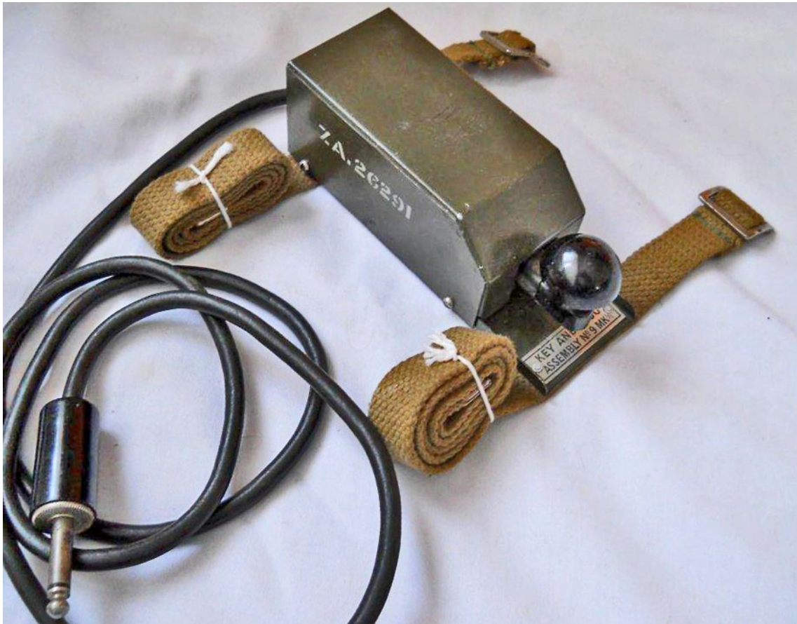
Key and Plug Assembly No. 9 Mk.1/1 ver. 4.3 was the tropicalised version of the No. 9 assembly. It was similar to ver. 4.2 except for having a different plug.
