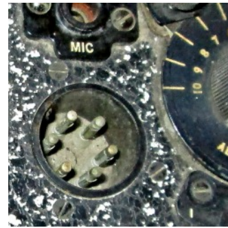
Close-up view of the set plug for connecting the key and plug assembly or the microphone.
