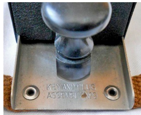
Front view of the No. 9 ver. 9.2 assembly. Note a differently shaped key knob and the designation stamped in the assembly base plate.
