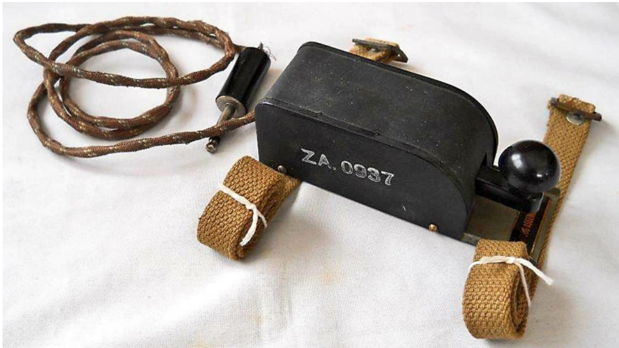
Key and Plug Assembly No. 9 ver. 3.3 was principally similar to ver. 3.2, but having a rounded protective cover.
