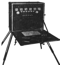
Figure 5.6: The BD-70 Switchboard
