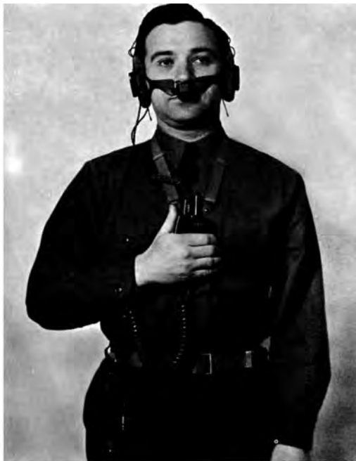
THROAT MIKE WORN BY A TANK CREWMAN, LEFT, AND LIP MIKE, RIGHT. Both could be used with radio or telephone.
