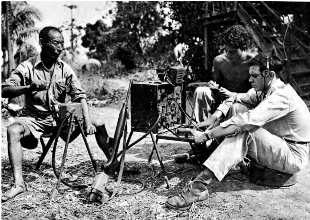
HAND-GENERATED RADIO, operated by men of the 988th Signal Battalion message center in Burma.
