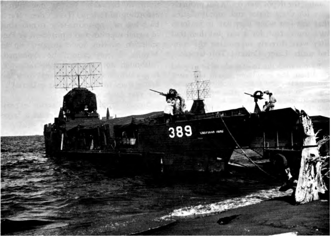
LW RADAR MOUNTED ON LST, NEW GUINEA
