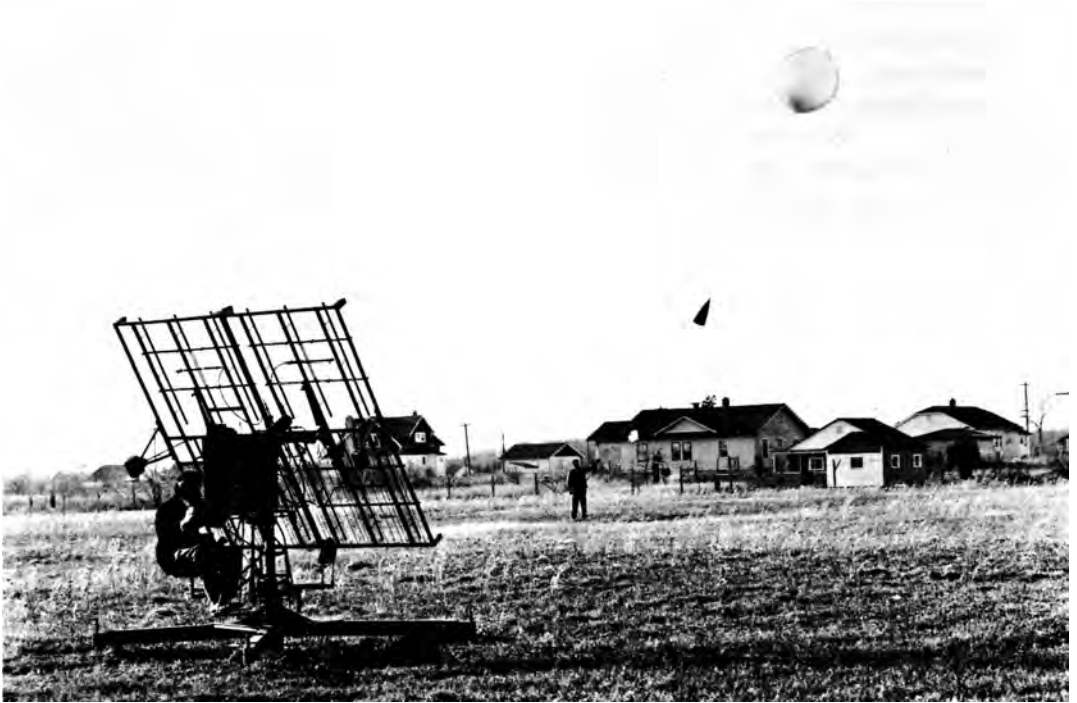
SCR-658 TRAINED ON RADIOSONDE AN/AMT-2 AT LAUNCHING
