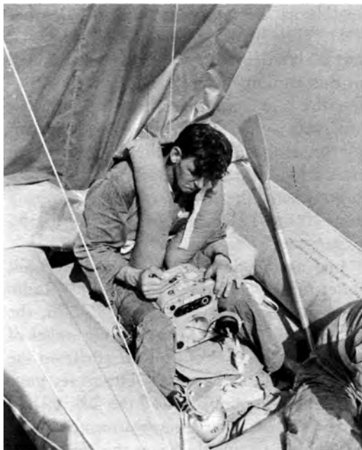
THE SCR-578, GIBSON GIRL RADIO. Distress signals were automatically transmitted when the crank was turned (left) and the antenna raised (right).
