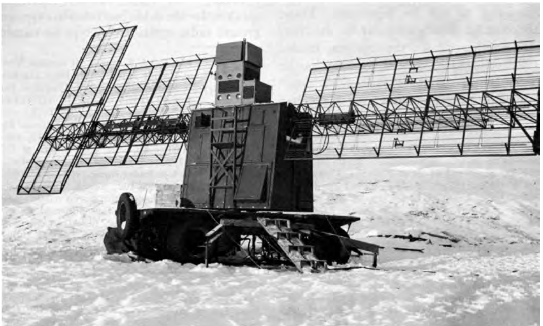
AIRCRAFT WARNING RADARS. The fixed SCR-271 on Ile des Pins in the Southwest Pacific (above) and the mobile SCR-268 in Greenland (below).
