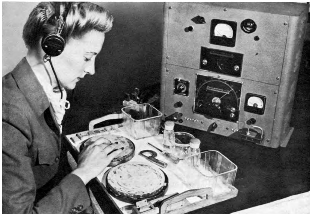
HAND-FINISHING A CRYSTAL. Crystals so finished were then checked electronically by the beat frequency method for accuracy.
