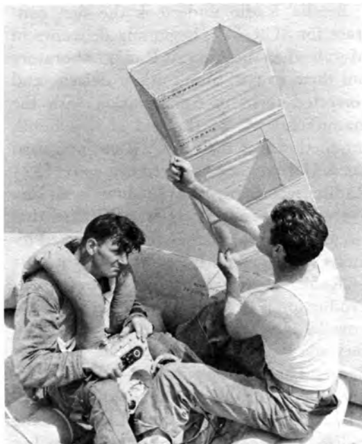
THE SCR-578, GIBSON GIRL RADIO. Distress signals were automatically transmitted when the crank was turned (left) and the antenna raised (right).
