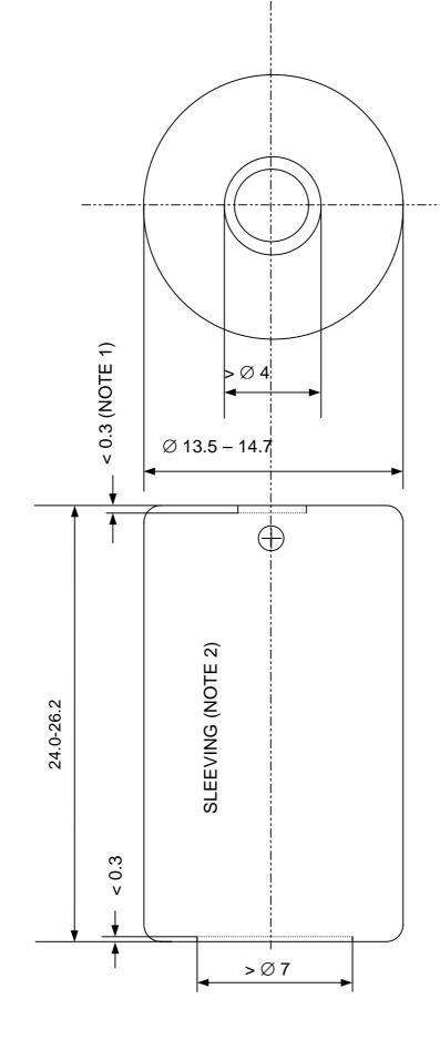
1. The positive and negative terminals shall be flush or proud of outer sleeving ideally, but may be sunken by a maximum of 0.3mm. NOTES:
