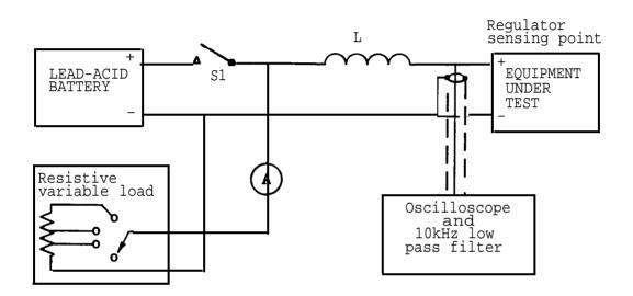
NOTE 1: S1...open - 'generator only' condition S1...closed - 'generator plus battery' condition
