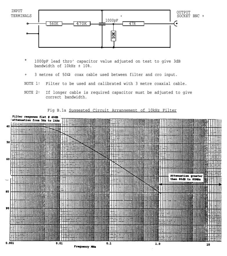
Fig B.1b Typical Frequency Response of 10kHz Filter + 3m Cable
