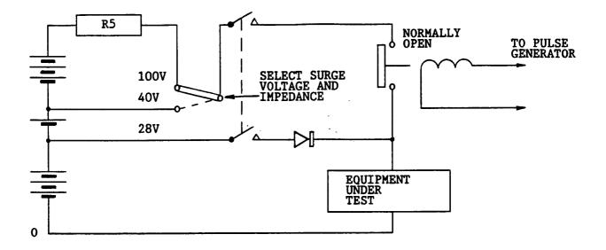
NOTE: Pulse generator produces 5 surges of 50ms duration at intervals of 1s between the commencement of each surge.
