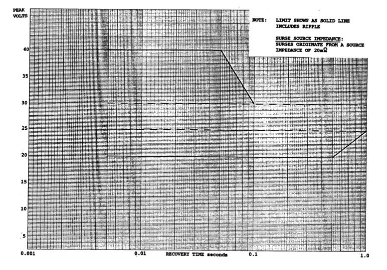
Fig 3 Surge Limit Generator Plus Battery Condition
