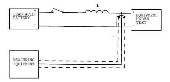
NOTE: L = 5µH for the simulated 'Generator Plus Battery' Condition or 50µH for the simulated 'Generator Only' Condition.
