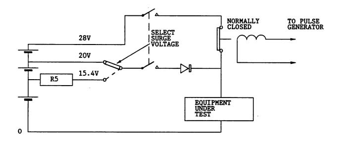
NOTE: Pulse generator produces 5 surges of 50ms duration at intervals of 1s between the commencement of each surge.
