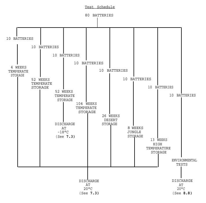
At least 8 batteries in any Sub-group of 10 and at least 71 batteries in the total of 80 batteries tested shall give not less than the minimum service output specified in 7.2, or 8.8.
